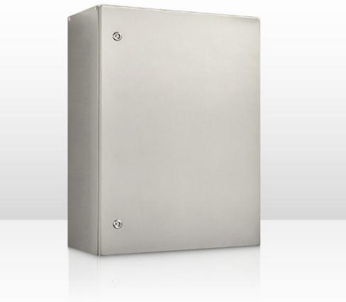
**Enclosure Body:** The robust monoblock body is fabricated using 1.5mm Grade 304L stainless steel. Flat face sealing surfaces are provided to increase seal life. Pre-fitted blind nuts are incorporated to accommodate mounts and accessory fasteners to eliminate drilling and retain IP rating. Integral device plate mounts and M6 earth studs are provided. Cutting, pressing and full continuous seam welding using precision automated manufacturing equipment ensures accuracy and consistent high quality.
